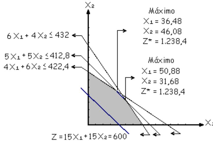
$$\begin{aligned} 5X_1 + 5X_2 &= 412,8 \\ 6X_1 + 4X_2 &= 432 \end{aligned}$$
