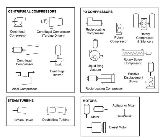
Figure 12.12 Compressors, Steam Turbines, and Motors
