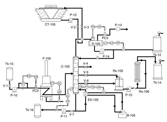
**Figure 12.3** *Process and Instrument Diagram (P&ID)*
